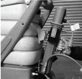
3. Connect your heater's inlet hose (#1 on page 11) to the machine's outlet quick disconnect (#6 on page 10).
