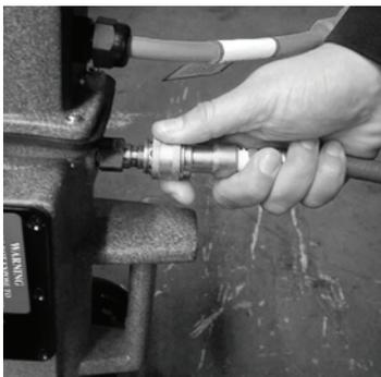
5. Connect the power cord on the heater to the female twistlock plug located on the rear of the R100H.
