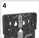
To manually unlock, push the locking mechanism toward the top of the dispenser. Note: This will leave the dispenser in an unlocked state until key is inserted to re-lock
