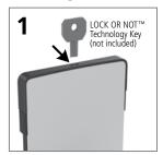
Lock the dispenser by aligning the key with the keyhole on the top of the dispenser and pushing down until a click is heard. Note: Once locked, dispenser will always require key to open, until LOCK-OR-NOT "auto-lock" functionality is manually
