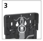
To manually remove the "auto-lock" function, unlock dispenser using key, remove refill, and take off white back plate of dispenser.
