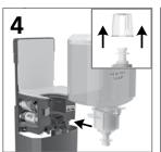
Remove the refill cap and push the new refill into dispenser until it clicks in place.
