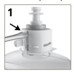
Insert a flat blade screwdriver into the slots on the refill collar and twist to separate the collar from the refill.
