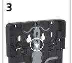
To manually remove the "auto-lock" function, unlock dispenser using key, remove refill, and take off white back plate of dispenser.
