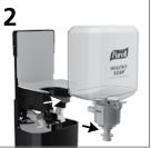
Push the **green** release button and remove empty refill.
