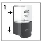
Open dispenser by pressing release buttons on the sides & slide the front cover down.
