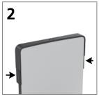
Check for a successful lock by pressing the release buttons on the sides of the dispenser to see if the front cover releases and slides down. Note: Once locked, the dispenser will remain in the locked state. To open a locked dispenser. insert the key into the keyhole and press down until the front cover is released.
