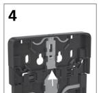
To manually unlock, push the locking mechanism toward the top of the dispenser. Note: This will leave the dispenser in an unlocked state until key is inserted to re-lock the system.
