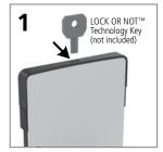
Lock the dispenser by aligning the key with the keyhole on the top of the dispenser and pushing down until a click is heard. Note: Once locked, dispenser will always require key to open, until LOCK-OR-NOT "auto-lock" functionality is manually turned off
