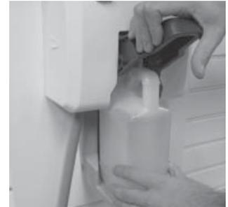
13. Raise handle on unit and insert product container onto shelf. Lower handle until it locks the bottle in place. Ensure bottle is aligned with chemical seal.
