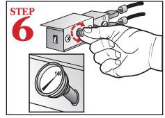
Adjust heater thermostat to 140F.
