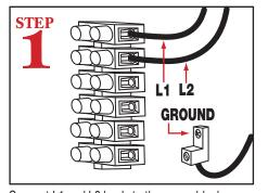
Connect L1 and L2 leads to the power block ground wire to ground lug.
