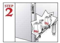
Connect water lines (hot 140F/160F) and (cold 75F) to water solenoid valves.
