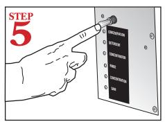
Flip power "on-off/flush" switch to "ON" position. Wash tank will automatically fill.
