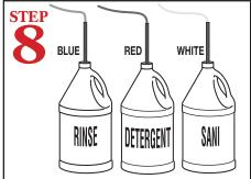
Insert tube stiffener with chemical tubing into corresponding chemical dispensers. PN: 10130.37
