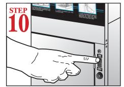
Start conveyor by flipping rocker switch to "ON" position.
