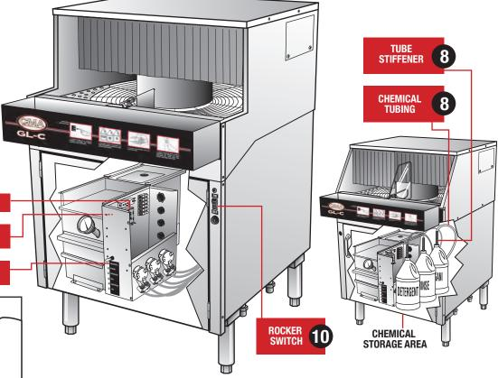
Adjust auto-fill timer to 10 seconds to set water level.
