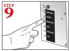
Push each of the chemical prime buttons and hold until the chemical feed tubes are full.
