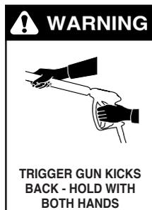
**WARNING:** Grip cleaning wand securely with both hands before starting. Failure to do this could result in injury from a whipping wand.
