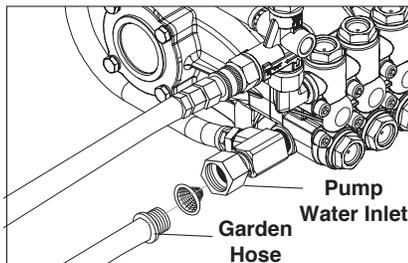
**STEP 7:** Check inlets filters, remove debris, then connect the garden hose to pump water inlet.
