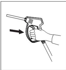
**STEP 4:** Press trigger to release water pressure.
