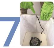
Install the new outer prefilter by aligning the prefilter seam with the power cord
