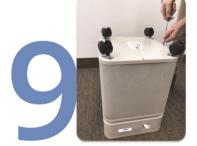
Replace the bottom cover & screw down tightly
