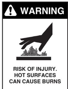
**WARNING:** Risk of injury. Hot surfaces can cause burns. Use only designated gripping areas of spray gun and wand. Do not place hands or feet on non-insulated areas of the pressure washer.
