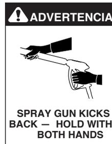
**WARNING:** Grip cleaning wand securely with both hands before starting. Failure to do this could result in injury from a whipping wand.
